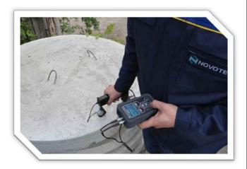
Measuring the strength and uniformity of construction materials by ultrasonic method NOVOTEST IPSM is designed for:
