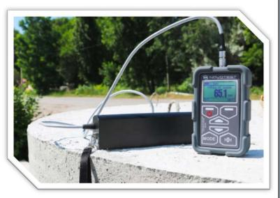
measurement of the protective layer, the estimate diameter;
