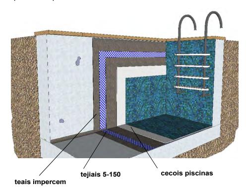
The product is applied for waterproofing of concrete walls, small-sized terraces, balconies, shower trays, waterproof coating of concrete surfaces subjected to external aggressions such as deicing salts, environments with sulfates, chlorides, waterproofing pools.
