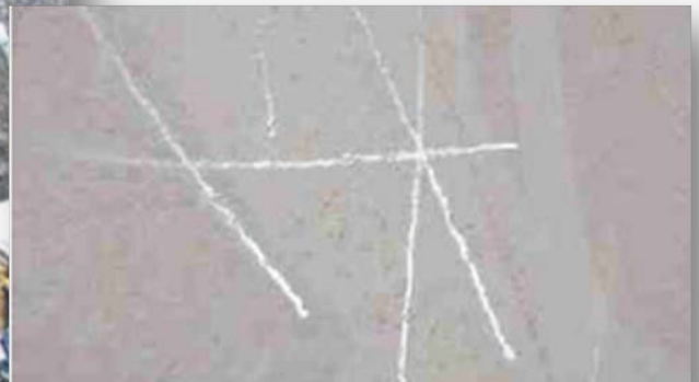
Photo Shows ZINGA “Liquid Galvanising”. Scratched with coin. Note: the pure zinc exposed.
