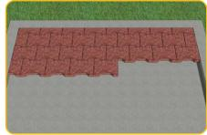
Cut tiles in a proper size and insert them in the blanks: use the special pieces "Cut V" or "Cut O" when possible
