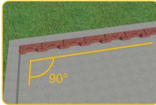
Install the whole tiles in a perpendicular horizontally and vertically direction
