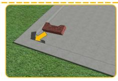
Start laying from one side of the walkway or from entrance of the carousel by placing a tile to the edge
