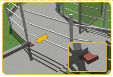
Install the first row of tiles up to the edge of the other side checking for a proper alignment and perpendicularity
