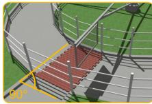
Start the second row with a tile of "Interlocking Cut O"
