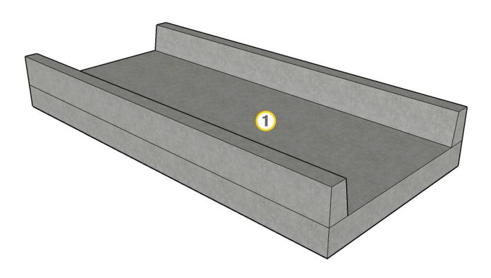
Add Krystol Internal Membrane (KIM) to the concrete mix in the bridge deck to protect the deck from de-icing salts. Refer to Application Instructions 1.11 to 1.15 — Use of KIM Admixture.
