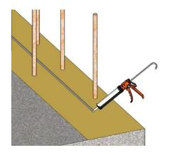
**IMPORTANT:** Krytonite needs to be placed at, or near, the center of the construction joint.
