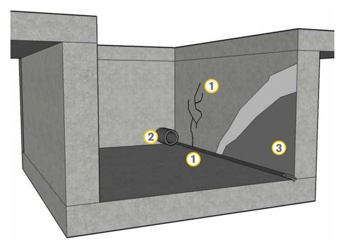
Negative side waterproofing for below grade structures where there has been no waterproofing or the waterproofing membrane has failed.
