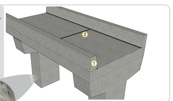
Krystol® chemically reacts with water and un-hydrated cement particles to form insoluble needle-shaped crystals that fill capillary pores and micro-cracks in the concrete and block the pathways for water and waterborne conteminants. Any moisture introduced over the lifespan of the concrete will initiate crystallization, ensuring permanent waterproofing protection.
