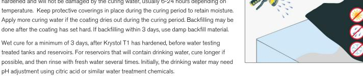
IMPORTANT: Freshly applied Krystol T1 must be protected from early drying, rain, frost and traffic. Once hardened it must be kept damp and wet cured for at least 3 days to develop its full properties. Longer curing periods are beneficial.
