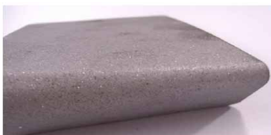
Figure 1. Results of Conical Mandrel bend test.
