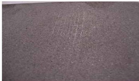
Figure 2. Results of cross-hatch adhesion test.
