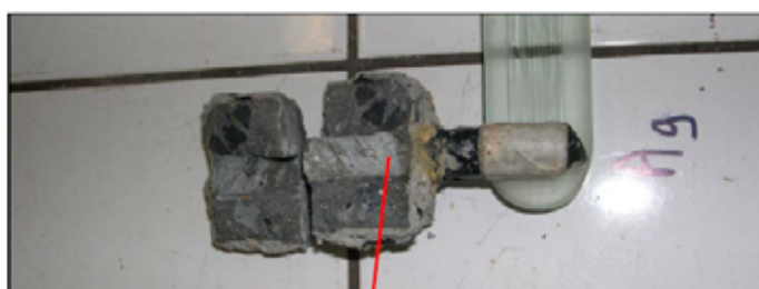
Thin layer of cement and Zinga on steel rod
