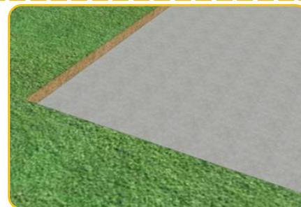
Apply the glue on the concrete surface with a notched trowel of 3 mm
