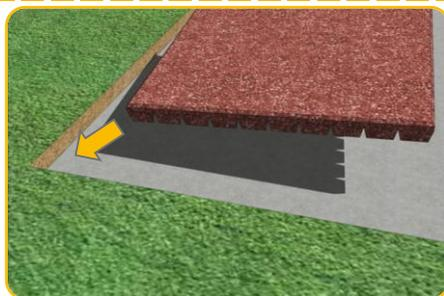
Install the first row of tiles to the edge of the other side checking for proper alignment and perpendicularity
