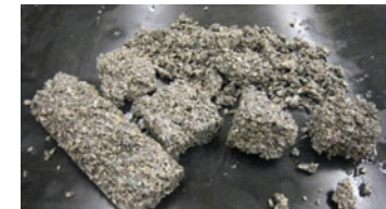
2 1/4" fiber at 7.5 lbs/cy retained almost complete integrity at 300 freeze-thaw cycles.
