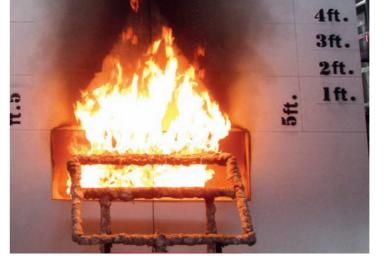
Senergy<sup>®</sup> - FOAMGLAS<sup>®</sup> EIFS system Fire test NFPA 285 approved
